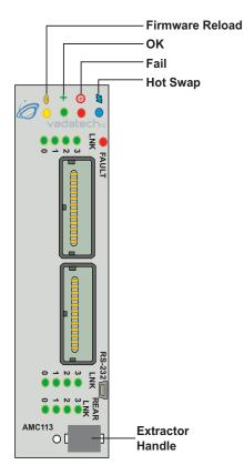
FIGURE 2. AMC113 Front Panel
