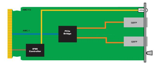
FIGURE 1. AMC113 Functional Block Diagram
